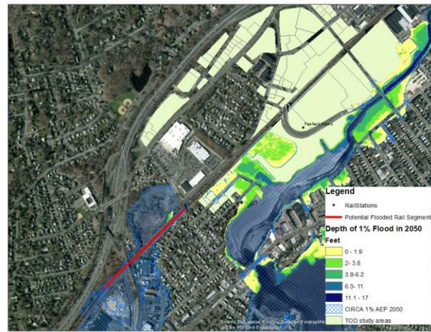
Figure: Map of 1% AEP in 2050 overlaid on the parcels studied around Fairfield Metro station. The red line highlights parts of the rail line also affected by the 1% AEP.
