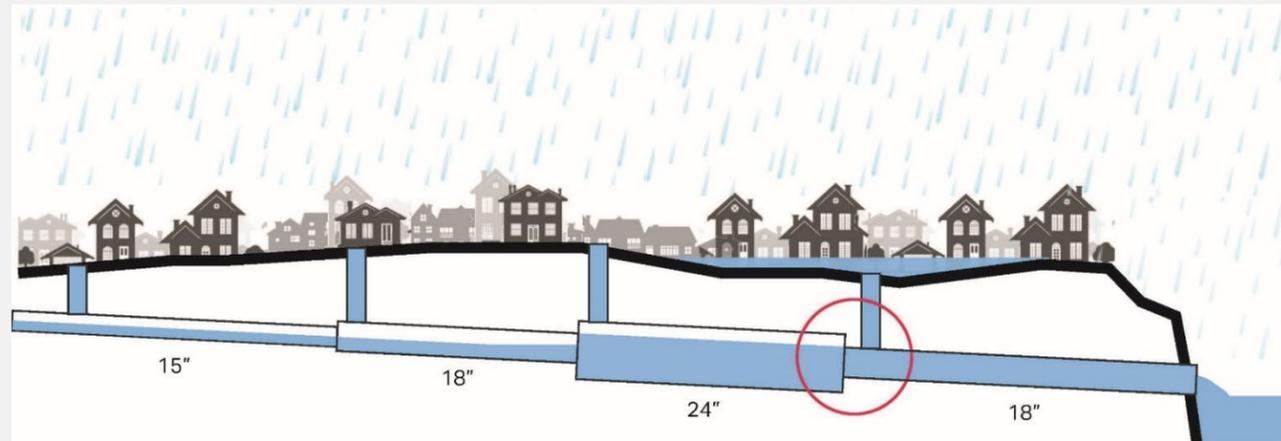
**Figure highlighting the drainage network downsizing concern. In a modern drainage system, the pipe diameter is designed to incrementally increase as you get closer to the outfall location to accommodate the continually increasing stormwater volumes.**
