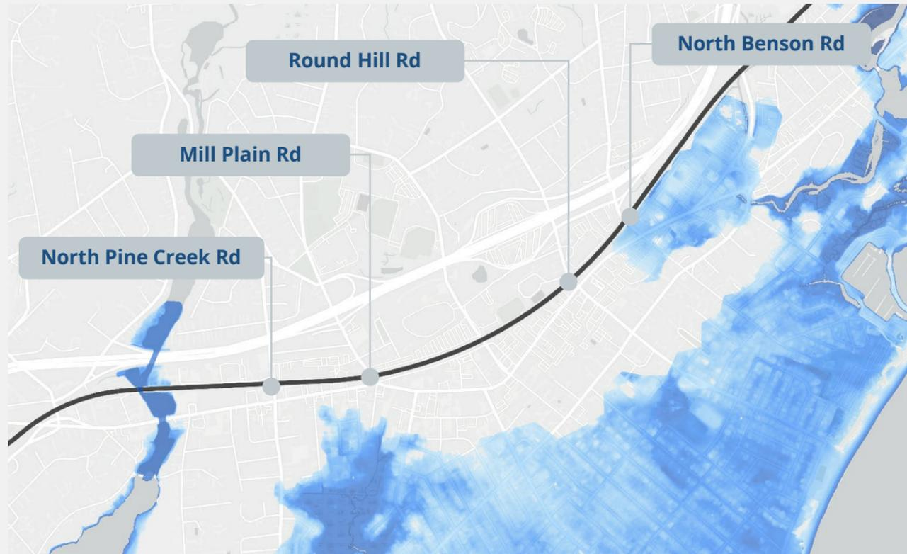
Extent of flooding and flood depth for a future 100yr storm assuming 20 inches of sea level rise. Under this scenario, the extent of the flooding extends further inland towards the underpasses and projected flood depths have increased. This future coastal flood scenario will likely further impact the ability of the existing drainage system to handle stormwater and will induce underpass flooding at lower precipitation levels.
