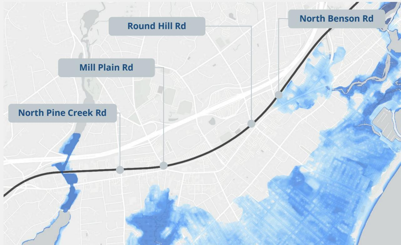
**Extent of flooding and flood depth for a current 100yr storm event. Under current conditions only the North Benson Rd underpass experiences inundation from a 100yr storm event.**
