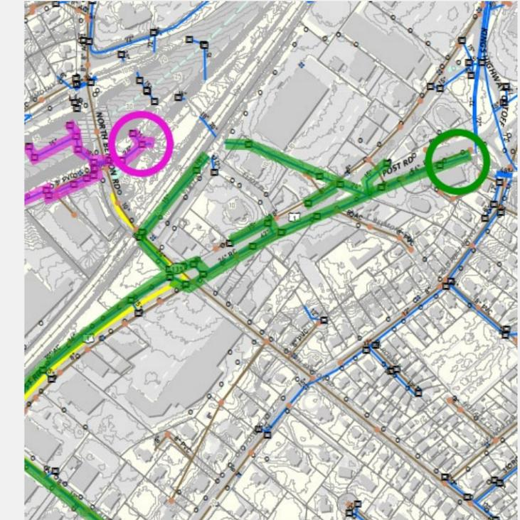
The underpass at North Benson Road is downstream of Round Hill Road within the same drainage system. The water collected from this area is eventually discharged into Ash Creek.
