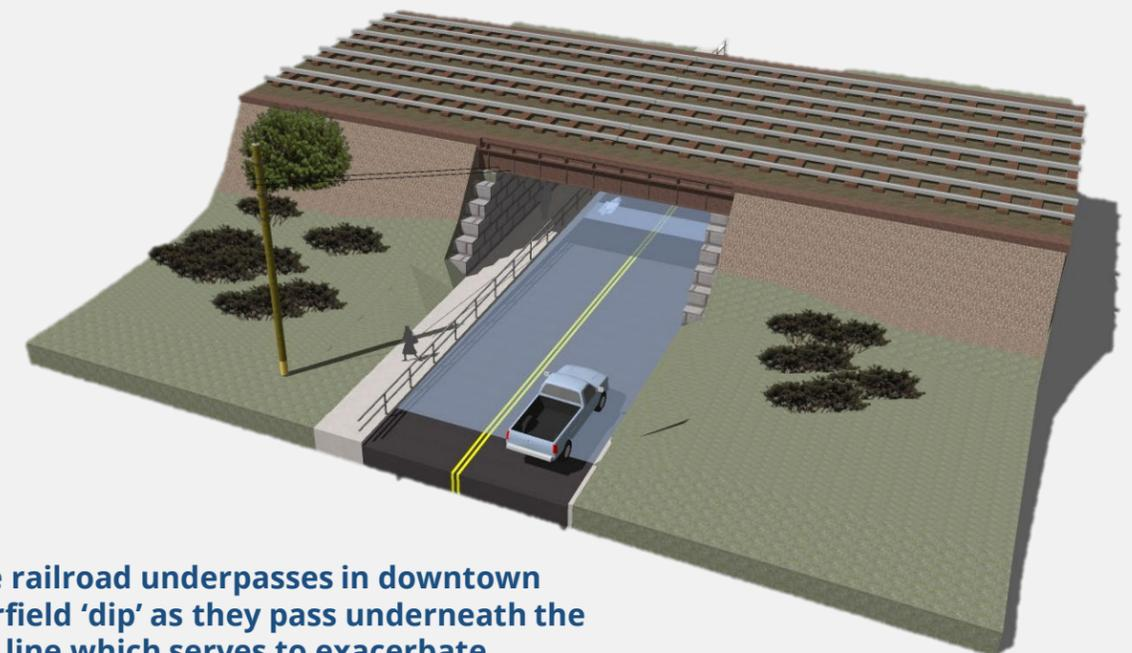
**The railroad underpasses in downtown Fairfield ‘dip’ as they pass underneath the rail line which serves to exacerbate drainage constraints and lead to accumulation of stormwater in the underpasses.**
