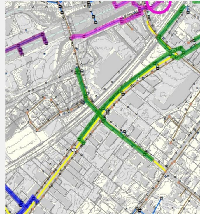
The drainage area around Round Hill Road is directed towards Ash Creek. The underpass at Round Hill Road shares a drainage network with the North Benson Road underpass as well as several additional side streets.
