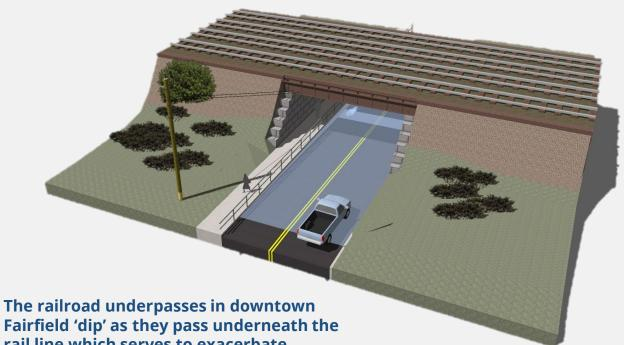
The railroad underpasses in downtown rail line which serves to exacerbate drainage constraints and lead to accumulation of stormwater in the underpasses.
