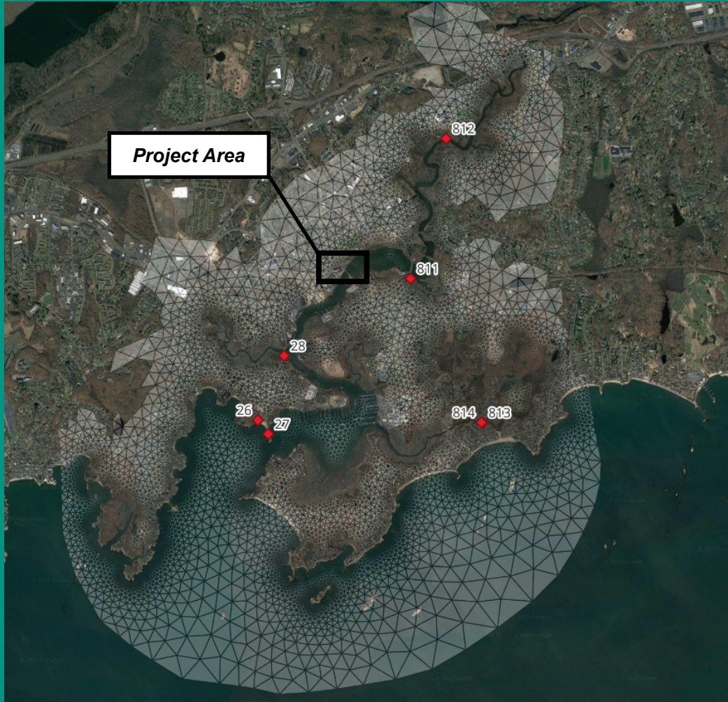
FIGURE 3. A visual representation of the Branford River flood modeling area. Red diamonds indicate the USGS high water mark (HWM) surveys from Superstorm Sandy.
