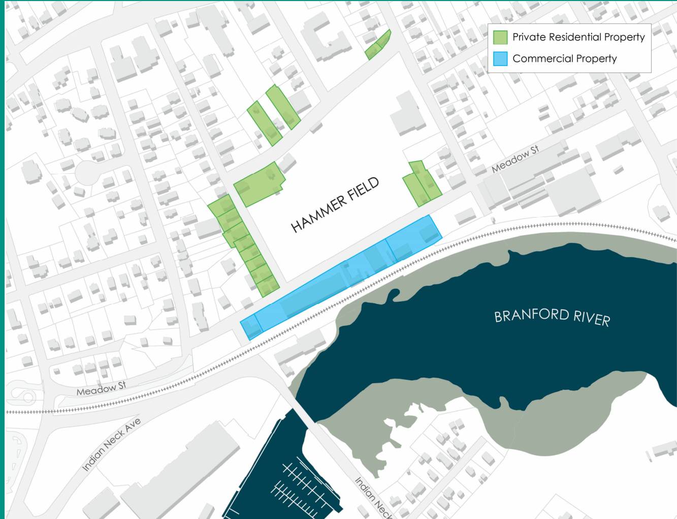
FIGURE 14: STRUCTURES POTENTIALLY PROTECTED FROM THE PRESENT DAY 100-YEAR STORM FLOODWATERS WITH THE CONSTRUCTION OF A FLOODWALL AND FLOOD GATE
